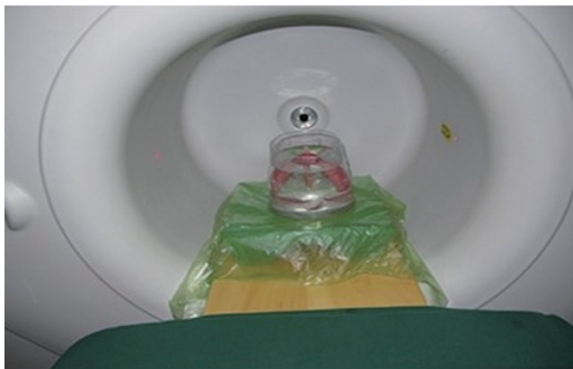
Fig. 3. NewTom 3G cone-beam computed tomography (CBCT). To obtain NewTom 3G CBCT scans, a dry mandible was placed in a plastic container containing water and positioned in a position similar to those used in clinical settings.
