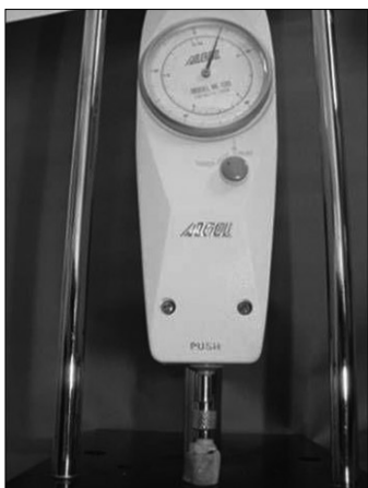
Fig. 1. A special loading device was designed to apply a constant load of 9.2 N to the ceramic discs.
