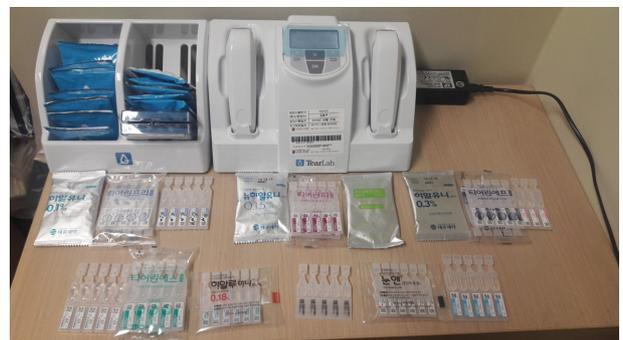
**Figure 1.** TearLab<sup>®</sup> osmometer and artificial tears used in this study. The artificial tears products were divided into five groups according to the type of ingredients and osmolality. For each group, three different products were selected and measured.
