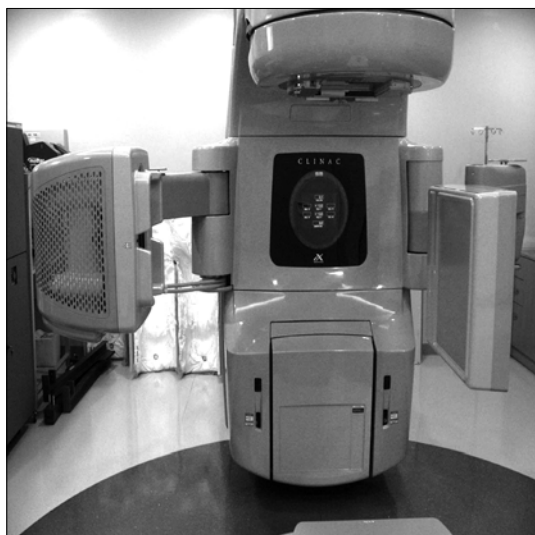
Fig. 1. On Board Imager (OBI) system installed on the conventional Linac. A X-ray generator is shown in the left side, and the detector is shown in the right side.
