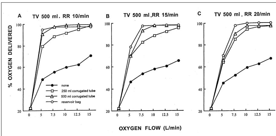
Fig. 4. The corresponding  $F_{D}O_2$  according to changes in the ventilator rate per minute at a fixed tidal volume (500 mL).
