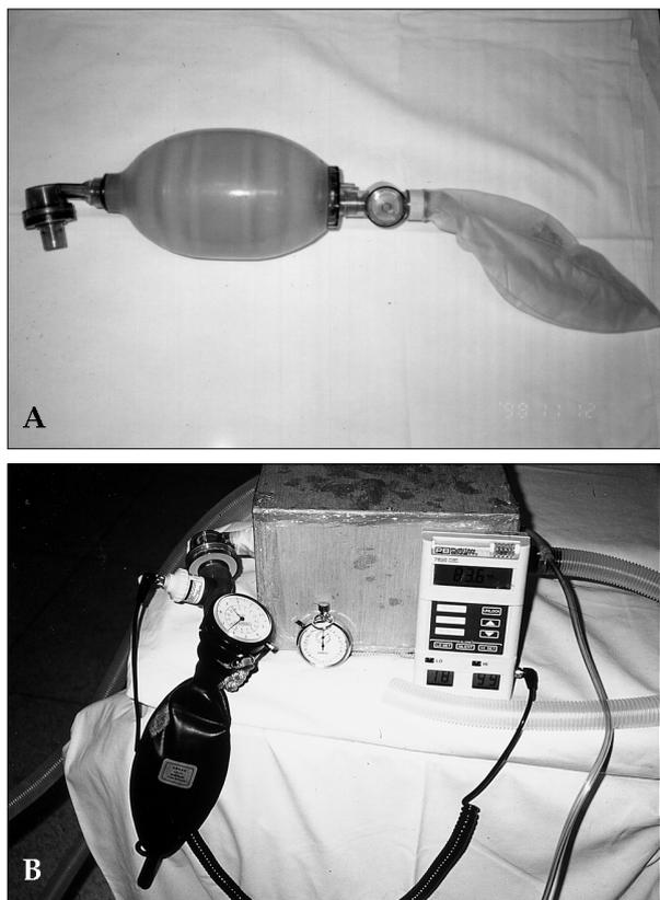
Fig. 1. The Laerdal resuscitator bag (A) and the sealed wooden box which encompasses the Laerdal resuscitator bag connected to a test lung, a spirometer and an oxygen analyzer (B).
