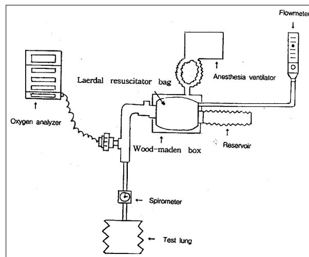
Fig. 2. Schematic drawing of the sealed wooden box with its connection to a test lung, a spirometer, an oxygen analyzer and a bellows of an anesthetic machine ventilator.
