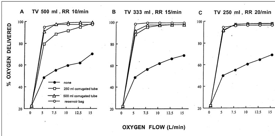
Fig. 3. The corresponding  $F_{D}O_2$  according to the changes of the tidal volume and the ventilator rate per minute at a fixed minute volume (5000 mL).
