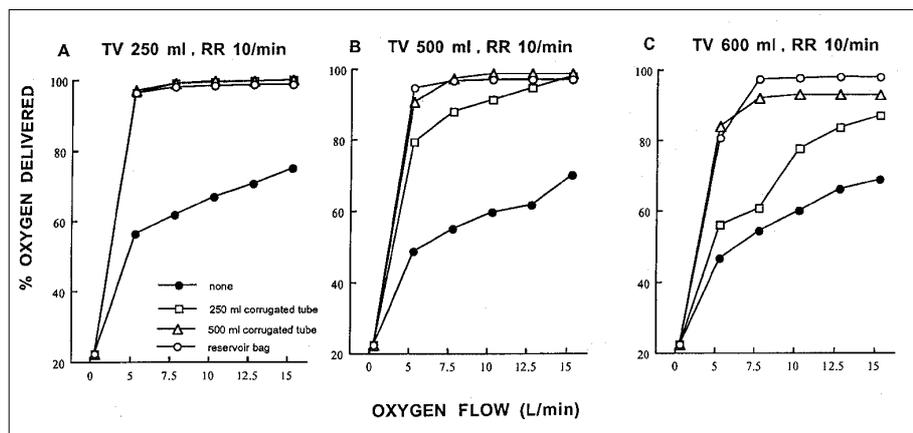
Fig. 5. The corresponding  $F_{D}O_2$  according to changes in the tidal volume at a fixed ventilator rate (10/min).
