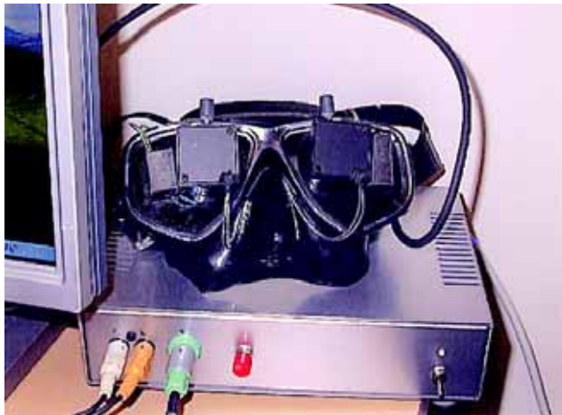
Fig. 1. Eye tracking system. The eye tracking system is composed of a head-mounted goggle and control box.
