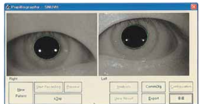
Fig. 3. Image analyses with pupil tracking software. A real-time, simultaneous, pupillary image is automatically targeted with a circle and was visible during testing on the computer screen.
