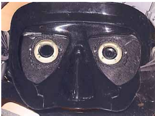
Fig. 2. Inner part of the goggle. The inner part of the goggle is composed of a CCD camera for image capture, two infrared LEDs for illumination, and four white LEDs for stimulation.
