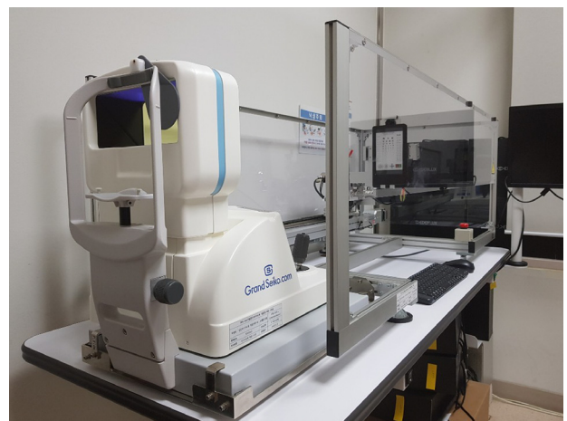
Figure 4. Auto refractometer (WAM-5500 Grand Seiko, Hiroshima, Japan). Objective refraction was measured under single viewing conditions. Moving target stimulate accommodation and auto refractometer measure amplitude of accommodation dynamically.
