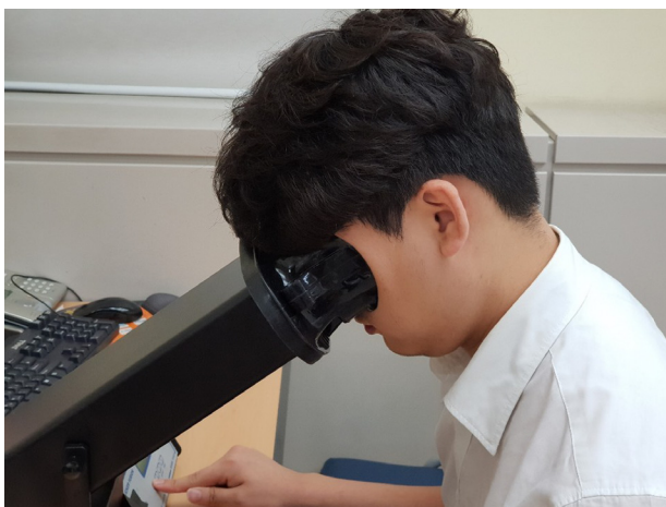
Figure 3. Flicker fusion frequency tester (Model 12021A, Lafayette Instrument Company, Lafayette, IN, USA). It can measure threshold frequency where a flickering light is perceived as continuous, defined as the critical flicker fusion frequency.
