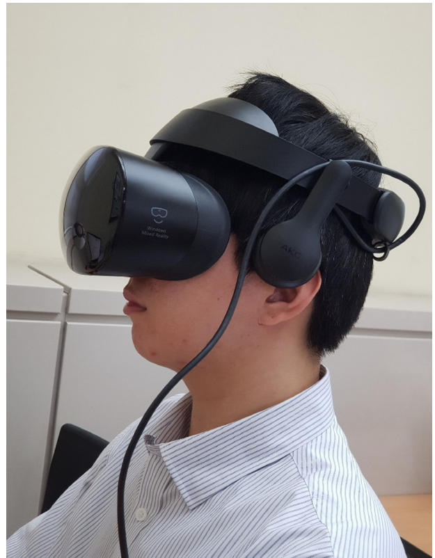
Figure 1. Head mounted display (HMD) based virtual reality (VR) display (XQ800ZAA-HC1KR, Samsung Electronics, Yongin, Korea). Subjects watched video for 10 minutes with VR device.
