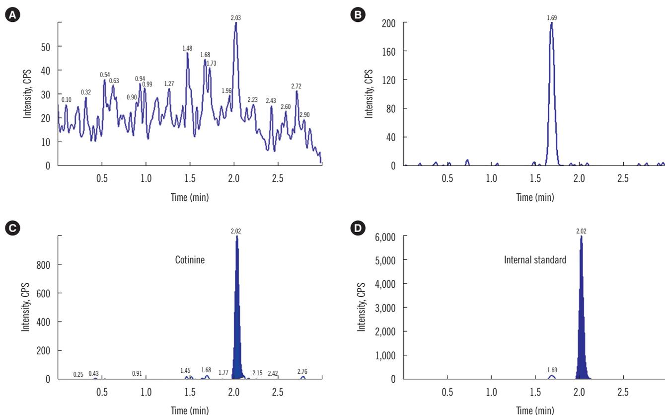
**Fig. 1.** Selectivity of serum cotinine using LC-MS/MS (A) Noise peaks (B) Front ghost peak (C) Cotinine (D) Internal standard (IS). No noticeable differences are observed in the chromatograms. Cotinine and the IS are separated from the noise peaks, and IS is sufficiently separated from the front ghost peak.
