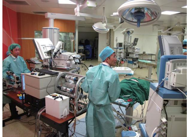
**Fig. 1.** Set-up of the entire Master and Slave TransEndoluminal Robot system, with the surgeon operating the master console of the robot at the left, and the endoscopist controlling the endoscope at the right.
