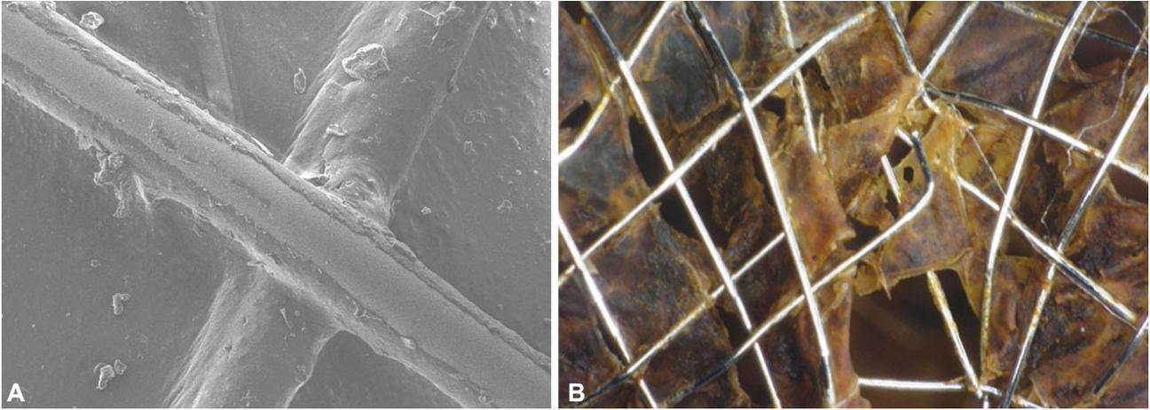
**Fig. 3.** Cracks in the covering membrane in the basic structure of the stent under long-term exposure to bile juice. (A) Scanning electron microscopy image. (B) Gross finding. Courtesy of S&G BioTech Inc.
