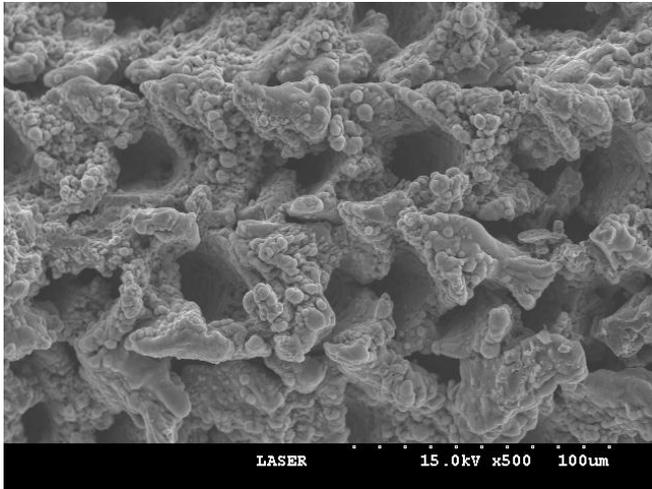
**Fig. 1.** FE-SEM image of the RBM-laser sample (original magnification,  $\times 500$ ). RBM-laser implant (experimental group) reveals precise porous structures dispersed uniformly throughout the implant surfaces. These porous structures are about 20–40  $\mu\text{m}$  in size. FE-SEM, field emission-scanning electron microscopy; RBM, resorbable blast media.
