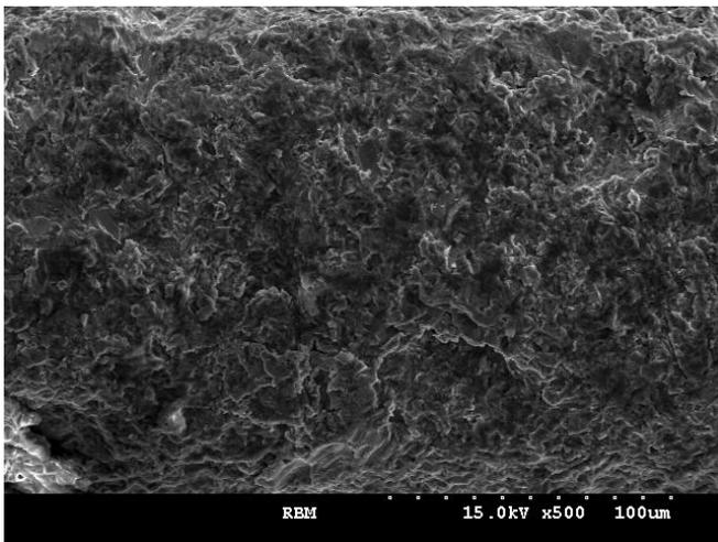
**Fig. 2.** FE-SEM image of the RBM sample (original magnification,  $\times 500$ ). RBM implant (control group) also reveals precise porous structures, however, these dispersed irregularly and its size is only 1–5  $\mu\text{m}$ . FE-SEM, field emission-scanning electron microscopy; RBM, resorbable blast media.
