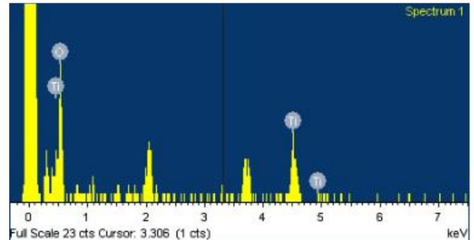
**Fig. 3.** EDS spectrum of the control RBM treated implant. The EDS analysis of RBM implant showed considerable surface contamination with several foreign elements. EDS, energy dispersive spectrometer; RBM, resorbable blast media; Ti, titanium; O, oxygen.
