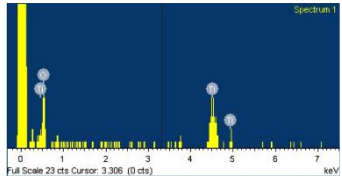
**Fig. 4.** EDS spectrum of the experimental RBM-laser treated implant RBM-laser implant showed a clean surface with Ti and O peaks. EDS, energy dispersive spectrometer; RBM, resorbable blast media; Ti, titanium; O, oxygen.
