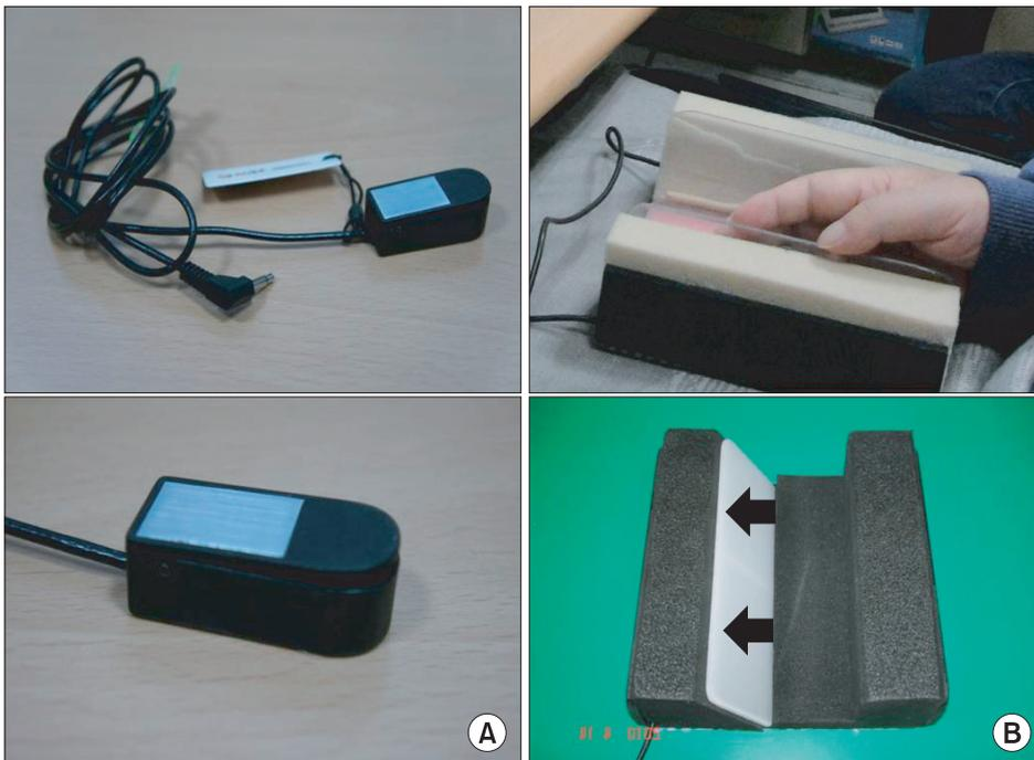
Fig. 4. (A) Micro light switch and (B) modified micro light switch is operated by the whole forearm.
