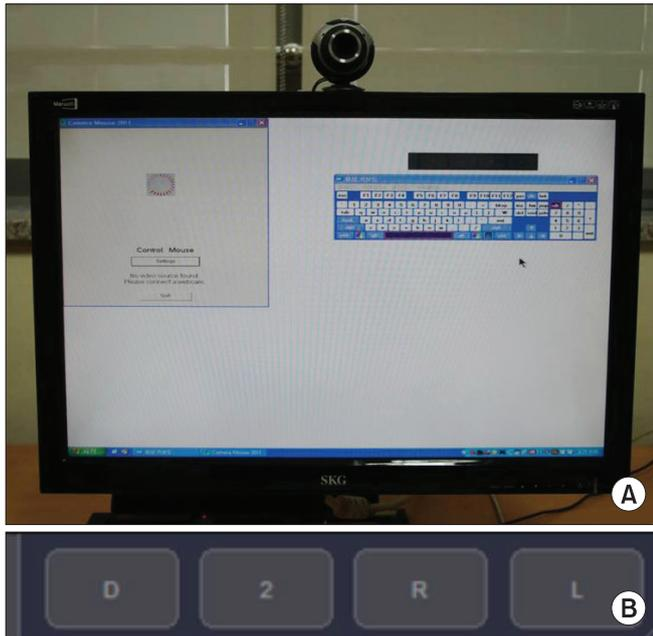
Fig. 3. (A) Combination of Camera Mouse, webcam, MintoClick 1.0, and screen keyboard and (B) MintoClick 1.0.
