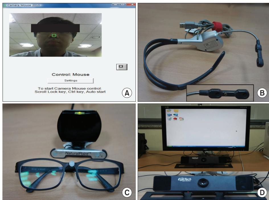
Fig. 1. The computer interfaces that sense the movement of a specific part of the body. (A) Camera Mouse, (B) Head Z mouse, (C) SmartNav 4AT, and (D) Eye-mouse4.
