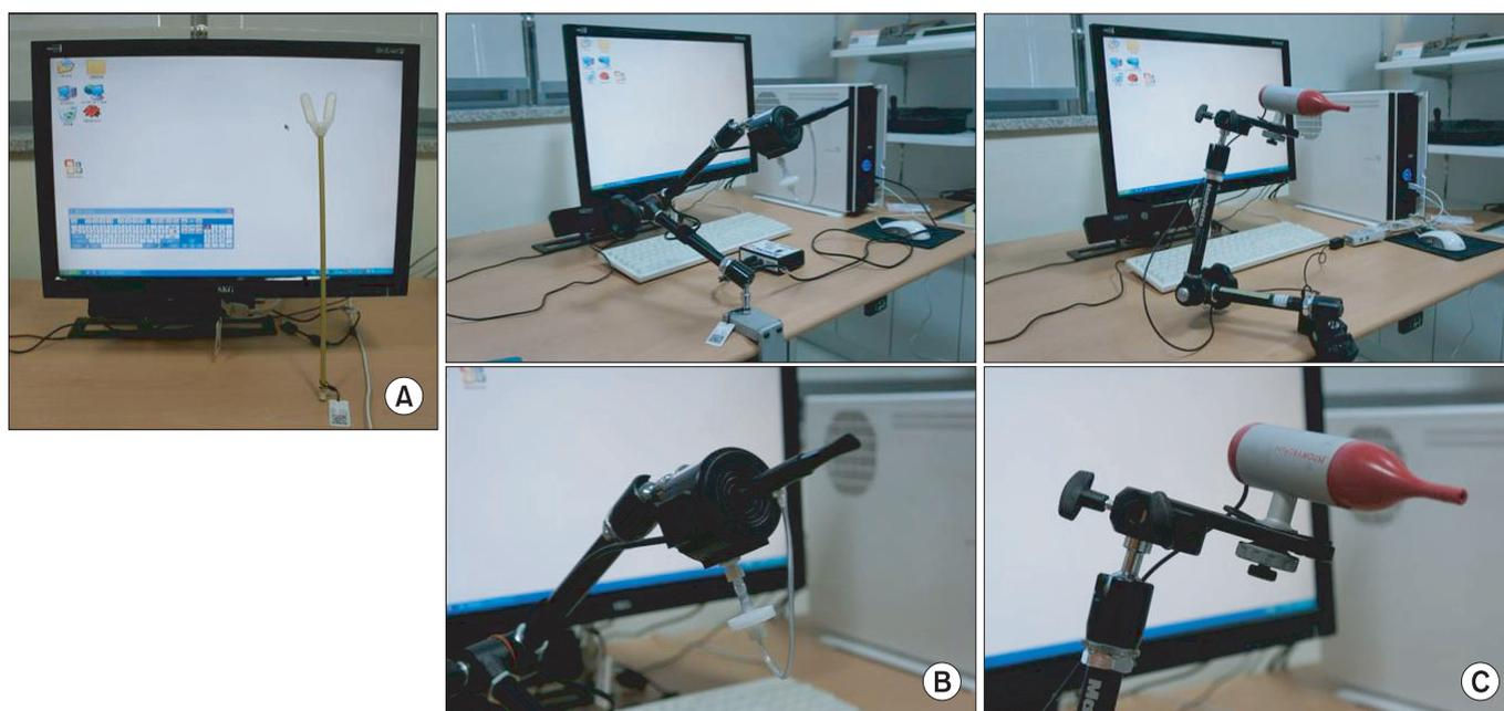
Fig. 2. The computer interfaces that are operated by the mouth. (A) Mouse stick and touch screen, (B) Jouse2, and (C) IntegraMouse.
