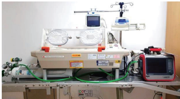
Fig. 3. The manufactured stretcher car which is specialized for the neonatal transport. It contains a transport infant incubator with battery, 2 oxygen tanks, a mechanical ventilator, a patient monitor, and an infusion pump.
