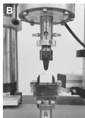
Fig. 2. 3- point flexural test. (A) Schematic diagram of specimens, (B) Universal testing machine.
