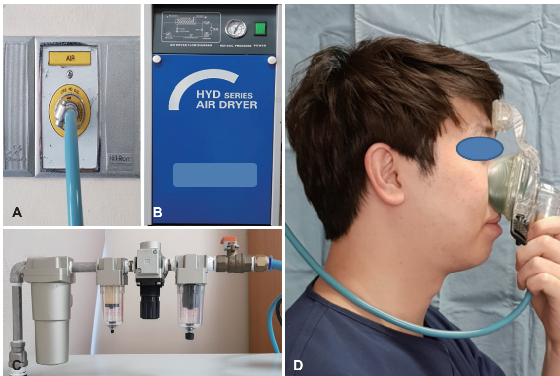
Fig. 1. Machinery for performing cold dry air (CDA) provocation test. We used the air for the medical use in the hospital (A). The refrigerator receives the air and generates a low-temperature air (temperature of about 0°C) (B). The filter and mist separator attached to the refrigerator filters dust and reduces the relative humidity of the air to less than 10%. The pressure regulator serves to regulate the air to be discharged at a constant pressure (C). The patient inhaled the CDA into the nose through the mask. This mask was originally made for continuous positive airway pressure treatment for obstructive sleep apnea, and we connected it to our CDA equipment to deliver CDA into patients' nose (D).
