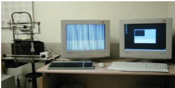
Figure 1. Head fixation device attached to head-mounted-display and CCD camera.
