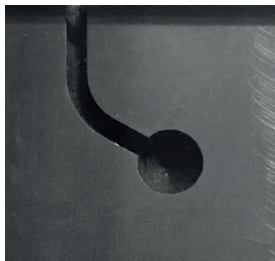
Figure 2. Artificial canal with single curvature that used in the present study.
