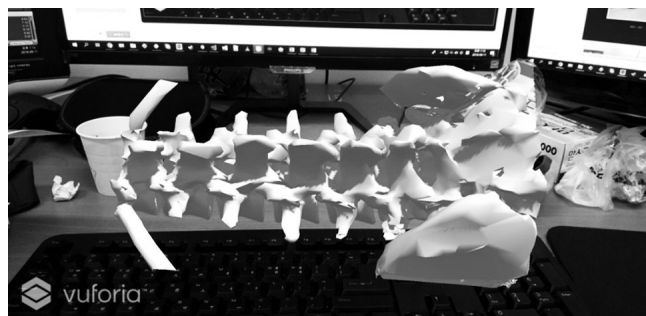
Fig. 3. Three-dimensional reconstructed model of the spine, which can be seen using a head-mounted device.
