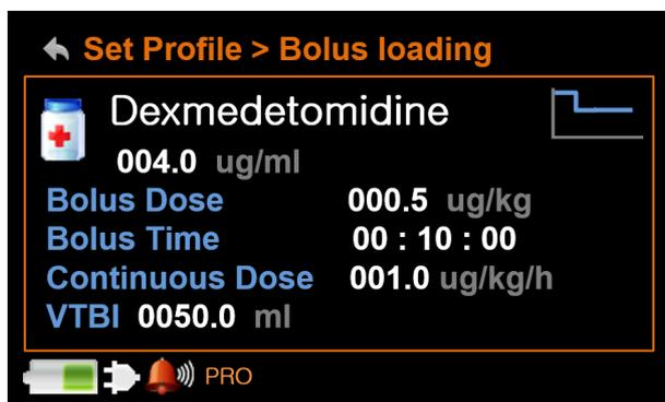
Fig. 2. This is the LCD screen of the syringe pump control panel. The bolus dose (5  $\mu\text{g}/\text{kg}$ ), which is the loading dose, is infused for 10 minutes, and the infusion rate is decreased to 1.0  $\mu\text{g}/\text{kg}/\text{min}$ . The VTBI (volume to be infused) is limited to 50 ml.
