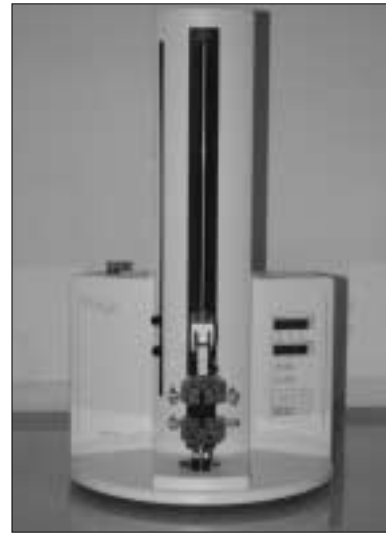
Figure 2. EZ test for microtensile bond strength test.
