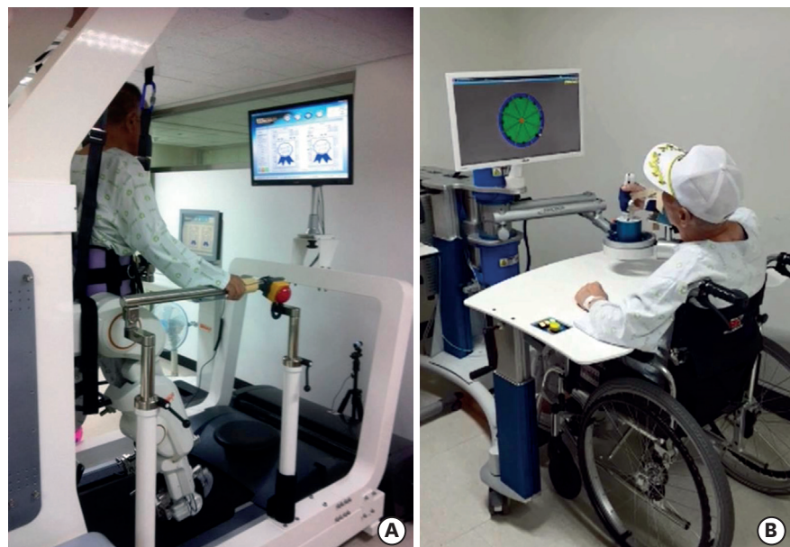
Fig. 1. (A) Exoskeleton robot-assisted gait rehabilitation using WALKBOT (P & S Mechanics, Seoul, Korea). (B) End-effector robot-assisted upper limb rehabilitation using MIT-MANUS/InMotion 2.0 (Interactive Motion Technologies Inc., Cambridge, MA, USA).
