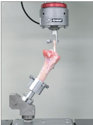
**Fig. 3.** Experimental set-up for load testing, showing tension being applied parallel to the tibial bone tunnel.
