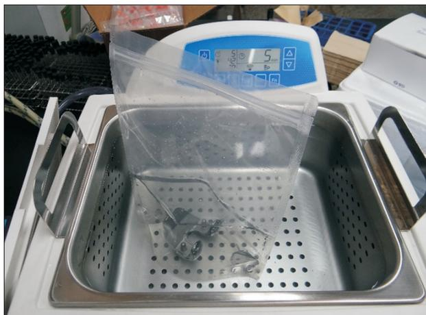
**Fig. 2.** The stomacher bag with 400 mL of saline and implant was subjected to sonication.
