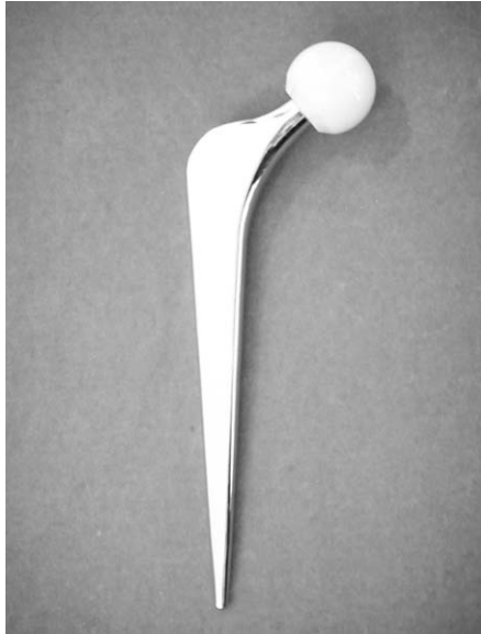
Fig. 2. Exeter ® stem has double tapered, collarless, polished wedge design. Once the stem is loaded, hoop stresses are set up with in the cement mantle as the stem engages, and creep takes place within the cement mantle.
