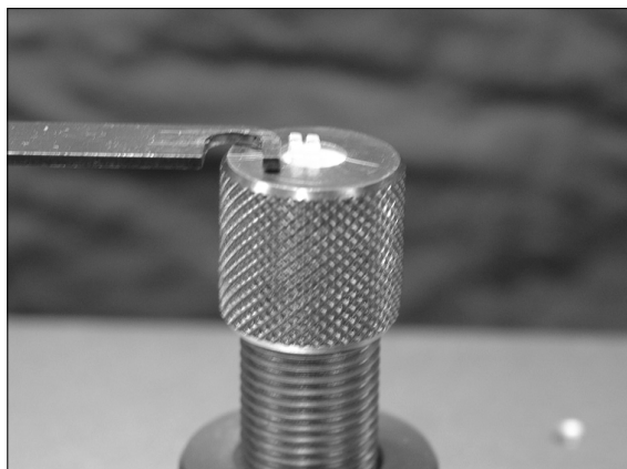
Fig 2. Application of shear debonding force.
