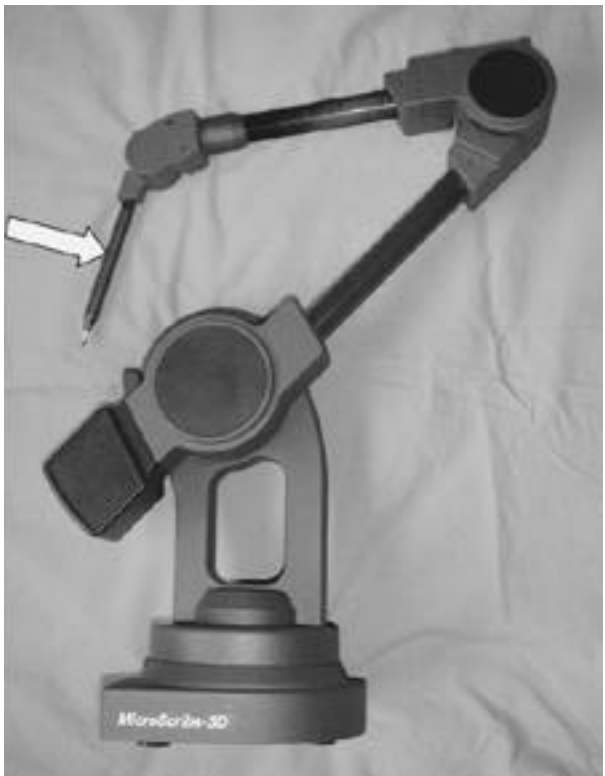
Fig. 1. A robot-arm type three-dimensional digitizer is shown. The stylus portion is arrowed.
