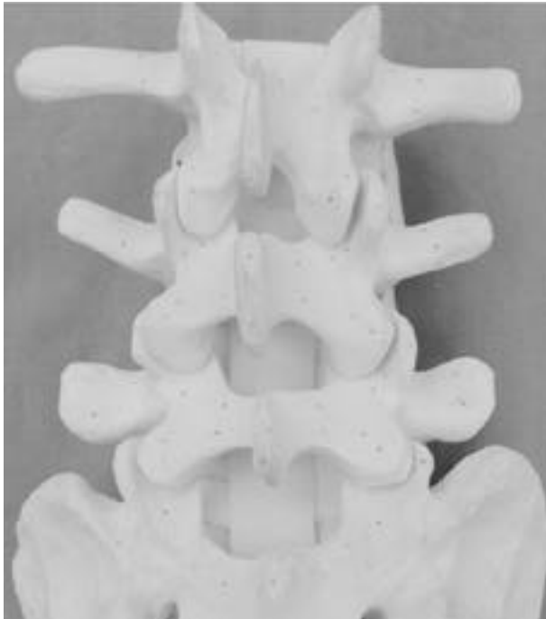
Fig. 5. A phantom made with a plastic lumbosacral bone model is shown. It was used for the accuracy test.
