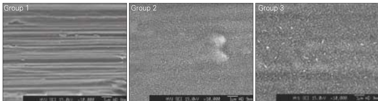
Fig. 4. FESEM (Field Emission Scanning Electron Microscope) findings of implant surface. Group 1: Machined, Group 2: Treated with alkali and heat in atmosphere, Group 3: Treated with alkali and heat in vacuum.
