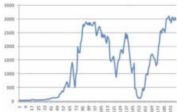
Fig. 3. Line analysis result of EPMA (Electron Probe Micro Analyzer) data of Ca at 6 week.
