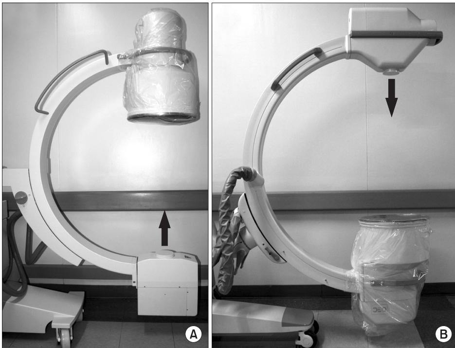
Figure 2. C-arm fluoroscopy with x-ray tube and image intensifier. (A) Typical C-arm fluoroscopy. (B) Inverted C-arm fluoroscopy.
