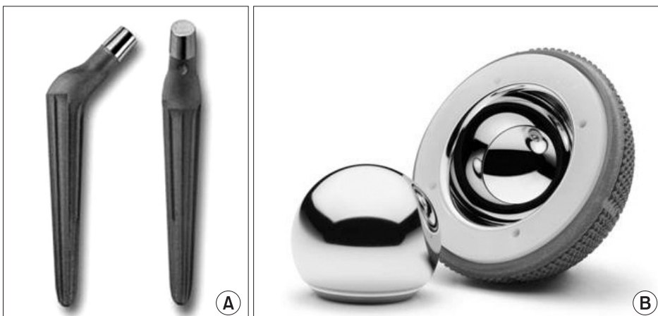
Figure 1. (A) Characteristics of the Wagner cone stem. It has a tapered angle of 5 degrees with eight sharp longitudinal ridges. It consists of a coarse blasted titanium surface for osseointegration. (B) Characteristics of the Fitmore cup. The outer surface of the implant consists of a 4-layered grid made of titanium. If press-fit stability is not achieved, screw fixation is necessary for optional stabilization.
