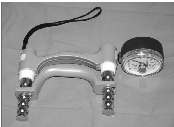
Fig. 1. Tool for measurement of grip strength, Jamar Hydraulic Hand Dynamometer (5030J).
