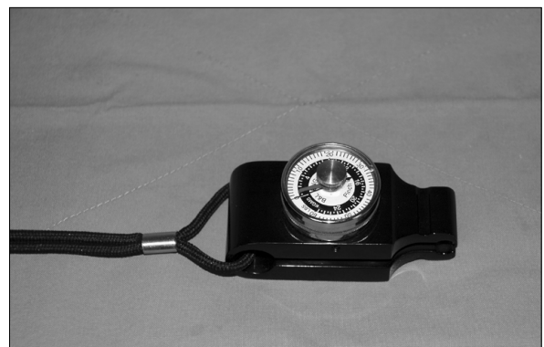
Fig. 2. Tool for measurement of pinch power, Jamar Pinch Gauge (PG 60).
