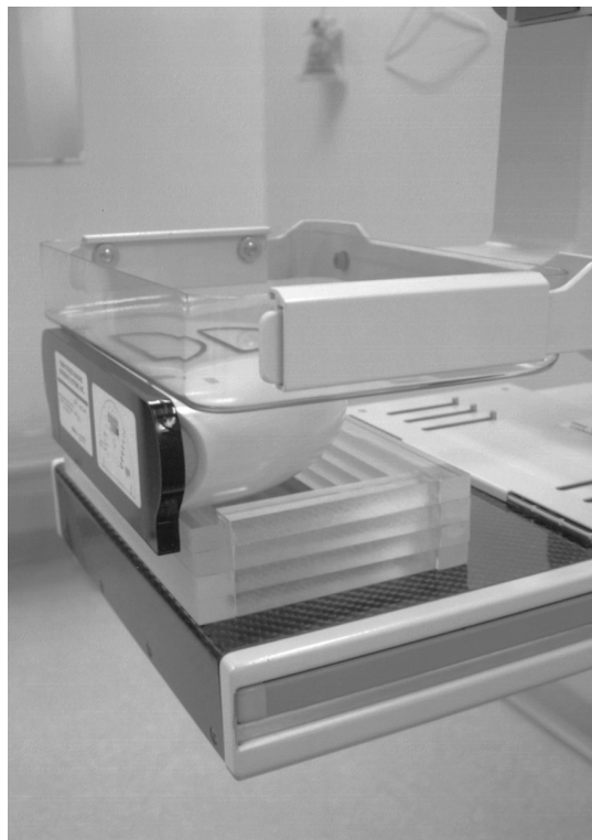
Fig. 1. A breast phantom is supported by multiple layers of acrylic blocks, each with a height of 10 mm. The true magnification factor is slightly higher, since most of the structure in the phantom (breast) will have a shorter FOD (Focus to Object Distance).
