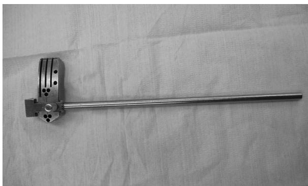
**Fig. 1.** Proximal resector with connecting instrument. This tibial AP axis synchronizer is composed of tail, caliper, and proximal tibial resector.
