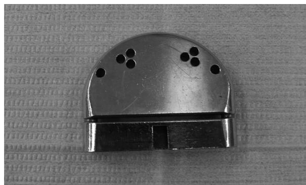
**Fig. 2.** The photo of distal femoral resector. Linker is composed of distal femoral resector and proximal tibial resector at knee extension position.
