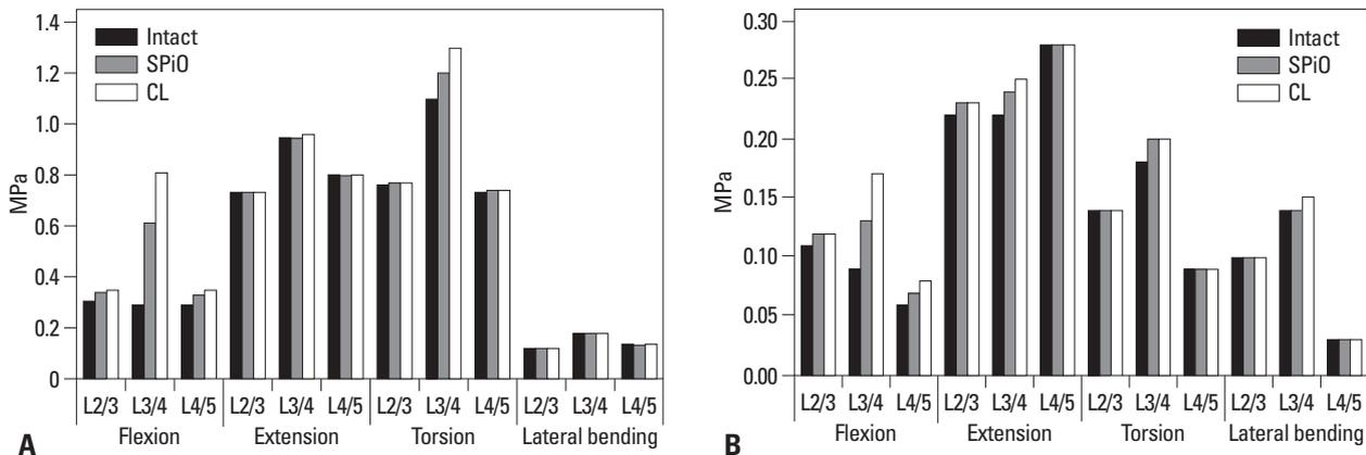
**Fig. 3.** Comparison of the maximal von Mises stress of the annulus fibrosus and the intradiscal pressure of the nucleus pulposus among three models. (A) Comparison of the maximal von Mises stress of the annulus fibrosus (MPa). (B) Comparison of intradiscal pressure of the nucleus pulposus.
