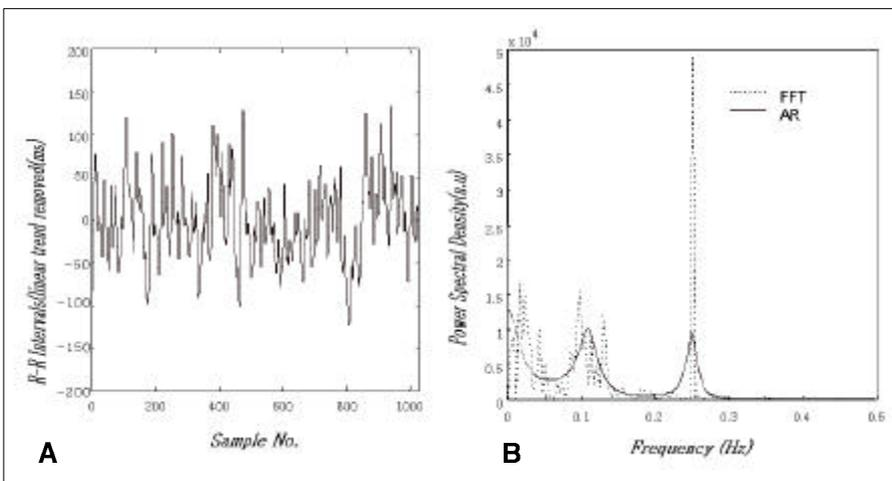
**Fig. 1.** Schematic outline of frequency domain analysis of HRV. (A) tachogram, (B) autoregressive power spectrum analysis
