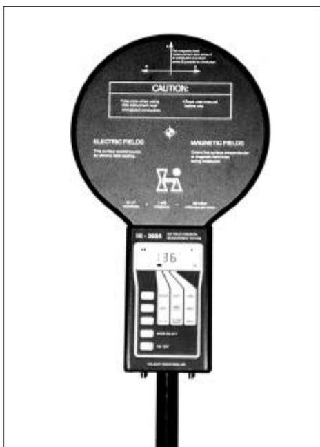
Fig. 1. Extremely low frequency (ELF) field strength measurement system
