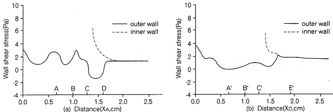
**Fig. 6.** Distribution of wall shear stress in steady blood flow. It is noted that the wall shear stress of outer wall is varying, initially. Then, it decreases approaching bifurcation, and represents its lowest value at the bifurcation site (B-C), prominent in the outer wall of the anterior descending artery (a). The highest value of wall shear stress is noted at the inner wall of bifurcation apex.
