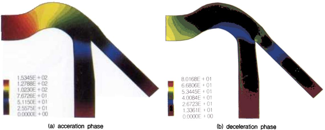
**Fig. 5.** The pressure contours of physiologic blood flow in the left coronary artery model (mmHg). Color legends and numbers represent the calculated value of pressure. The numbers are represented as exponential form. It is noted that the pressures of the inlet are 153.45, and 80.16 mmHg in acceleration (a), and deceleration phase (b), respectively. There is no definitive abrupt change, but it is skewed to the axial flow direction in deceleration phase.
