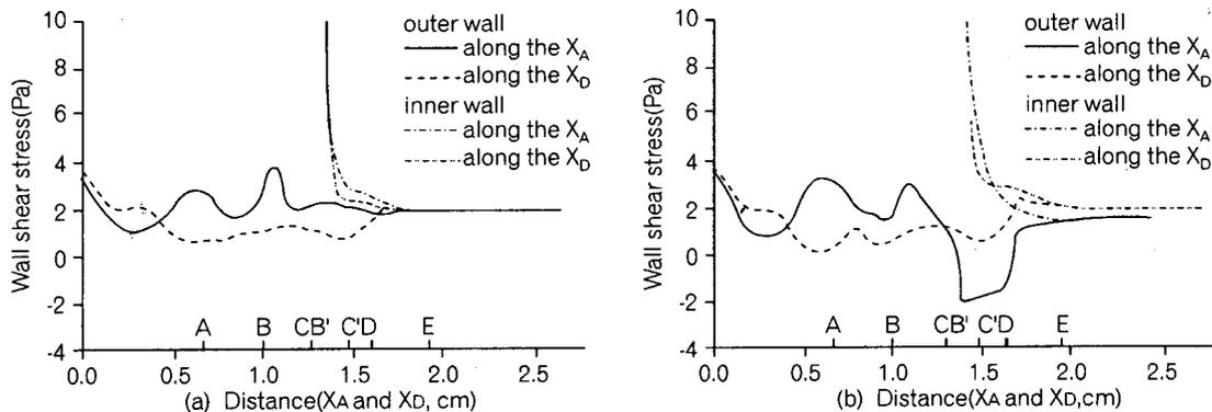
**Fig. 7.** Distribution of wall shear stress in physiologic pulsatile blood flow. It is noted that the wall shear stress of outer wall is varying, initially. Then, it decreases approaching bifurcation, and represents its lowest value at the bifurcation site (B-C), prominent in the deceleration phase (b) of the outer wall of the anterior descending artery. In acceleration phase (a), there were no definitive abrupt changes in the outer wall from inlet to both branching arteries.
