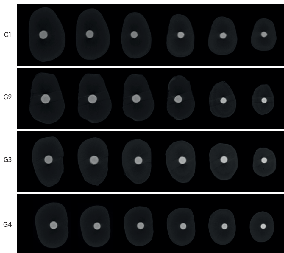
Figure 4. Two-dimensional slices from micro-computed tomographic scanning of axial cross-sections of obturated root canals from coronal third to apical third level (left to right) in each experimental group. Group 1 (G1), GP/AH; Group 2 (G2), BCC/AH; Group 3 (G3), GP/BCS; Group 4 (G4), BCC/BCS. AH, AH Plus; GP, gutta percha; BCC, bioceramic-impregnated gutta percha cone; BCS, bioceramic sealer.
