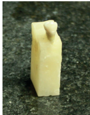
Figure 1. Specimen mounted in acrylic block.
