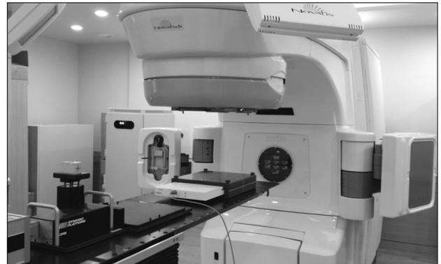
Fig. 1. System for the DQA process with the MapCHECK2 measurement and the dynamic moving phantom for the accurate control of gating window time.
