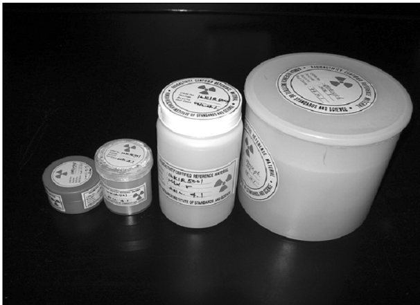
Fig. 2. The photography of various CRMs for the efficiency measurement of various measuring containers and the detection system.
