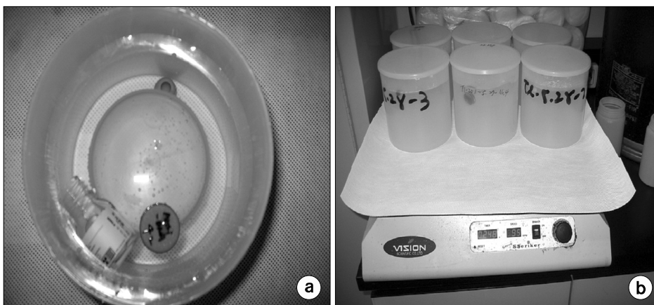
Fig. 1. The photographs of Marinelli beaker containing the radioactive waste from nuclear medicine department. (a) Marinelli beaker with radioactive wasted container and saline solution, (b) the dissolution and diffusion of radioactive nuclide in saline solution using a stirrer.
