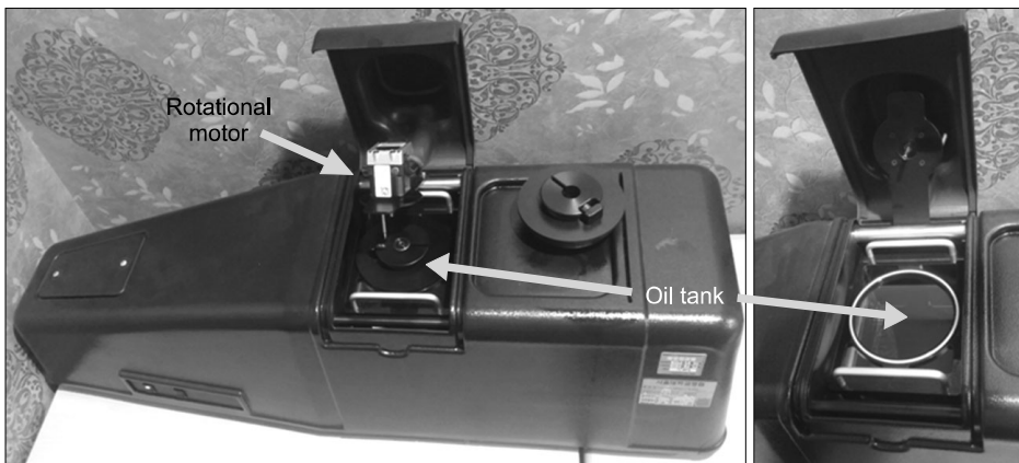
Fig. 2. Vista TM optical CT scanner. dove tail on the gel can be attached to the rotational motor, and gel body is immersed into oil tank.
