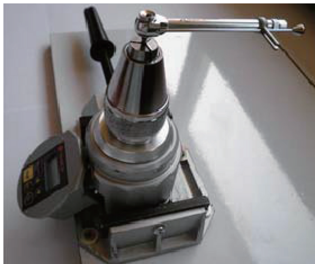
Figure 4. After connecting the devices to the appropriate drivers, they were clamped in a stable torque gauge.
