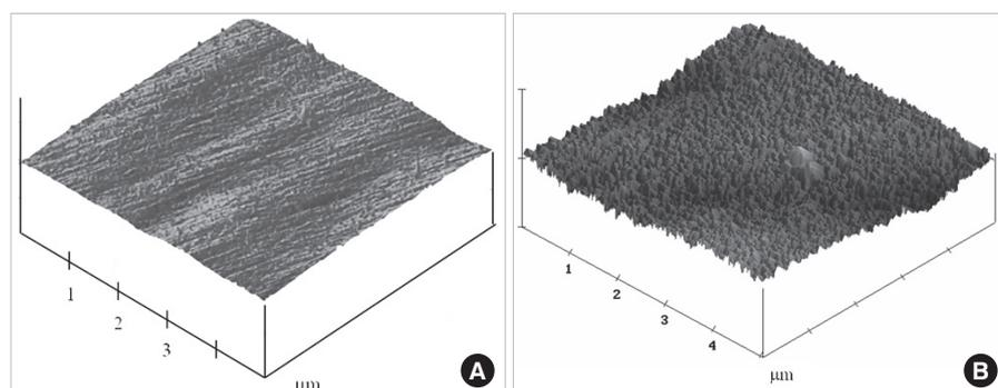
**Figure 3.** Atomic force microscopy (AFM) analysis of (A) commercially pure titanium (group cp-Ti) and (B) alkali- and heat-treated titanium-8tantalum-3niobium (group AHT). Three-dimensional AFM images (5 × 5 μm) showed nanoscale roughness on the group AHT surfaces. The surface topography of group AHT had more spike shape than the group cp-Ti.
