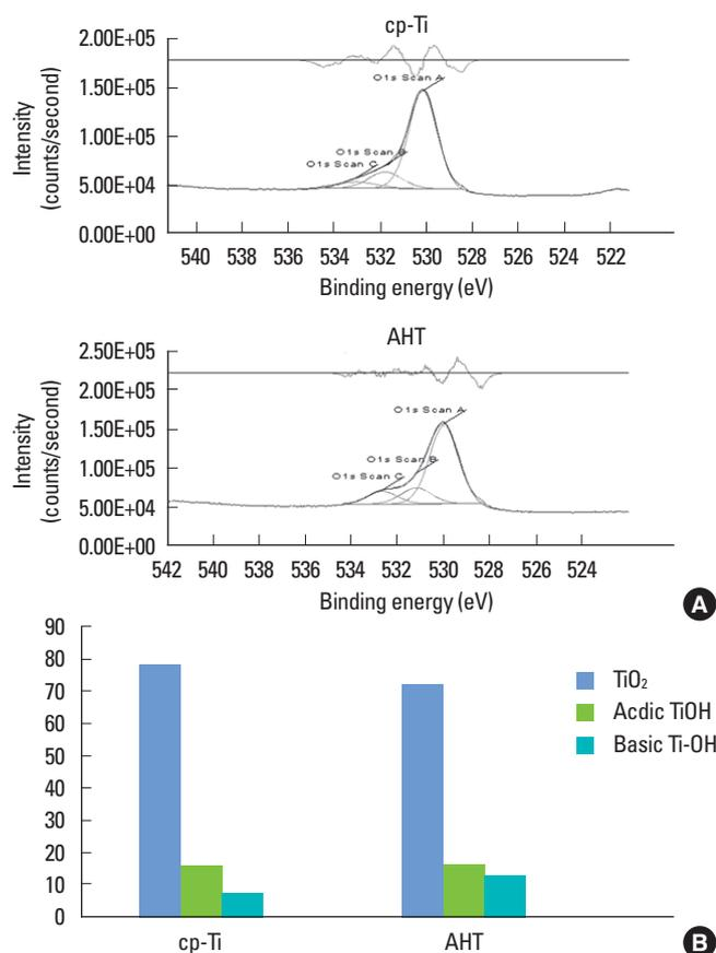
**Figure 2.** X-ray photoelectron spectroscopy analysis. (A) O1s spectra and (B) percentage of three oxygen species for commercially pure titanium (group cp-Ti) and alkali- and heat-treated titanium-8tantalum-3niobium (group AHT). Group AHT showed increased amount of hydroxyl groups on the surface layers. TiO<sub>2</sub>: titanium dioxide, TiOH: acidic titanium hydroxyl group, Ti-OH: basic titanium hydroxyl group.
