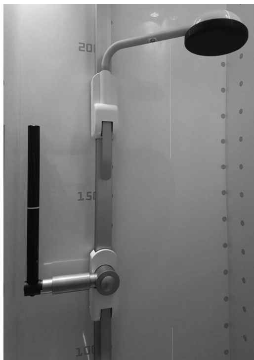
Fig 2. An X-ray tube and a sensor installed at a 90° angle, taking images from all sides at the same time, and a safety bar and a device fixing the patient's head in place while the image is obtained.
