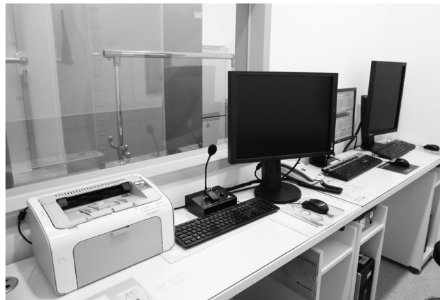
Fig 3. A separated EOS station protected from the X-ray. The length and angles of the obtained images are measured and reproduced as 3-dimensional images by the EOS software at this station.
