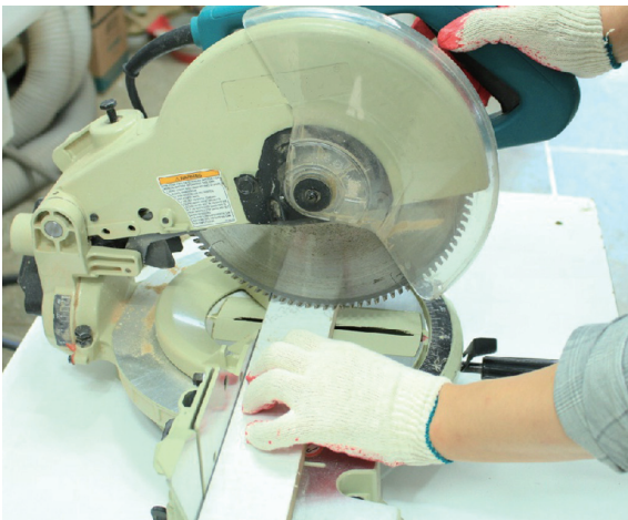
Fig. 3. Typical hand position while operating a hand-mounted saw. We can expect the non-dominant hand, which is pushing the object, to be injured.
