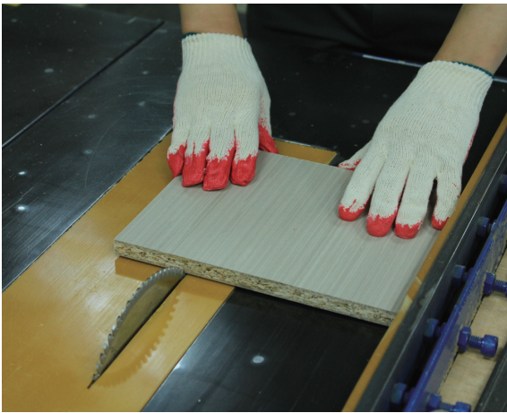
Fig. 2. Typical hand position while operating a table-mounted saw. We can expect the dominant hand, grabbing an object, to be injured.
