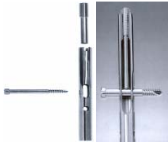
Fig. 1A. Proximal part of Interlocking-Compression (IC) nail composed of locking holes, screw and a compression screw. 1B. Feature of dynamic compression generated by the compression screw via the proximal dynamic locking screw.
