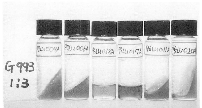
Fig. 2. Lot No. of 96LU018 and 96LU017 remain unchanged in liquid state at 25% of glue concentration.
