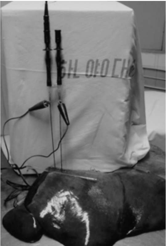
Fig. 1. Dual probes designed by our group. Two expandable radiofrequency electrodes are connected by electric cable after each insulator was removed.
