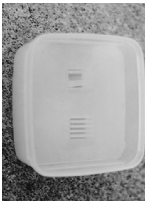
Fig. 1. Phantom was designed with 3% agar-gel block containing empty slits to form magnetic susceptibility difference. The air spaces were 1.6 mm in thickness, 25 mm in width, and 20 to 25 mm in depth with 1.6 mm spacing.
