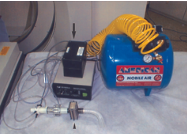
Fig. 1. Lung volume controller comprised of mouth piece part (arrowhead), transducer part (arrow), and personal computer part (not illustrated). This system was built by gathering each ready-made part.
